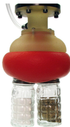
(e) Positive Pressure Universal Gripper Based on the Jamming of Granular Material (from [10])
