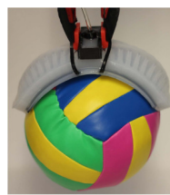
(b) 2018 Soft pneumatic gripper embedded with stretchable electroadhesion (from [40])
