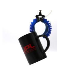
(c) 2018 Soft gripper with gecko-inspired adhesive (from [41])
