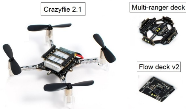
Figure 2 - Crazyflie 2.1 and expansion decks
