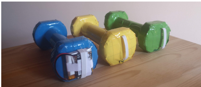
Figure 3. The three dumbbells of our prototype and the IMU which can be attached to any of the weights.
