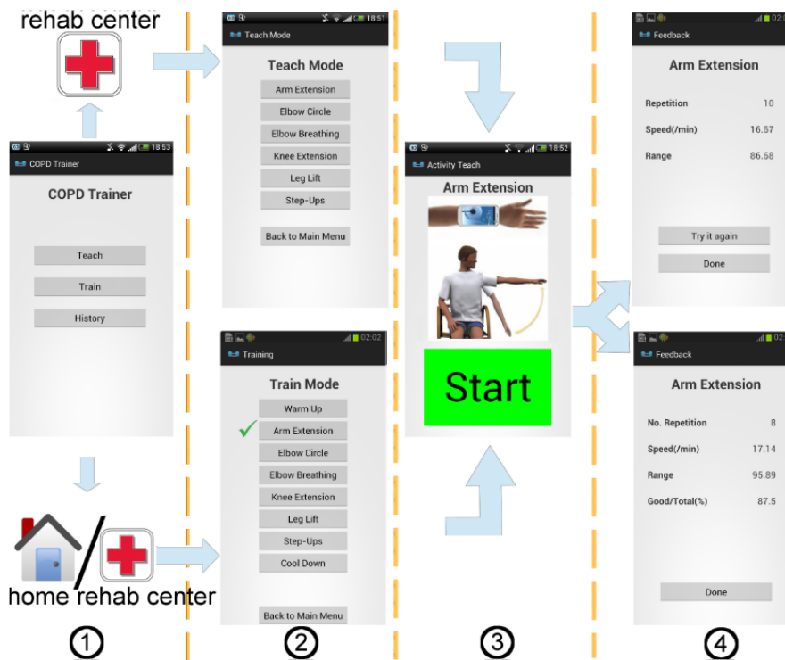
Figure 2.2: COPDTrainer training approach: The smartphone app is meant to enable individual training options of a patient, besides the training with therapists. (1): Patient/therapist selects Teach-mode or Train-mode. (2): Select an exercise, here Arm extension. (3): Begin exercising after pressing start. (4): After exercising different summary screens are shown, depending on the operation mode.
