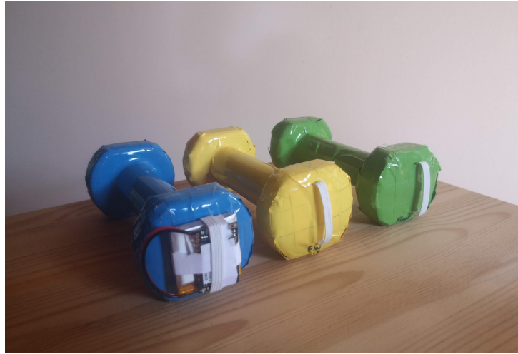
Figure 3.3: The three dumbbells of our prototype and the IMU which can be attached to any of the weights.
