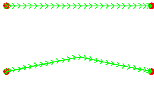
Figure 4.16: Trajectory before (top) and after (bottom) k_c is set from 0 to a positive value.
