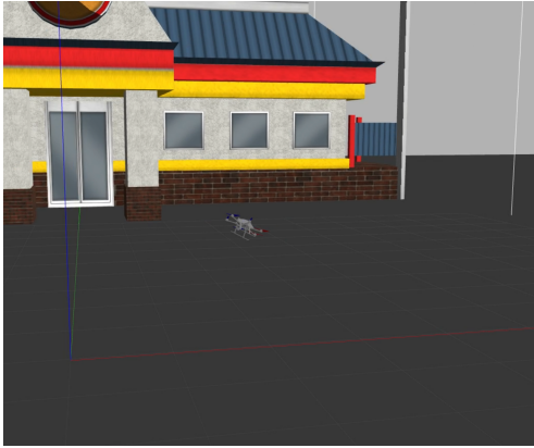
Figure 6.67: Vehicle assuming an attitude to accelerate from the initial hovering position
