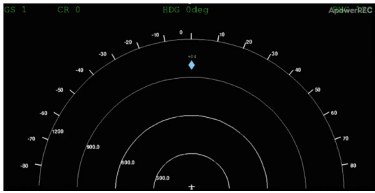
Figure 6.70: Intruder aircraft is detected.
