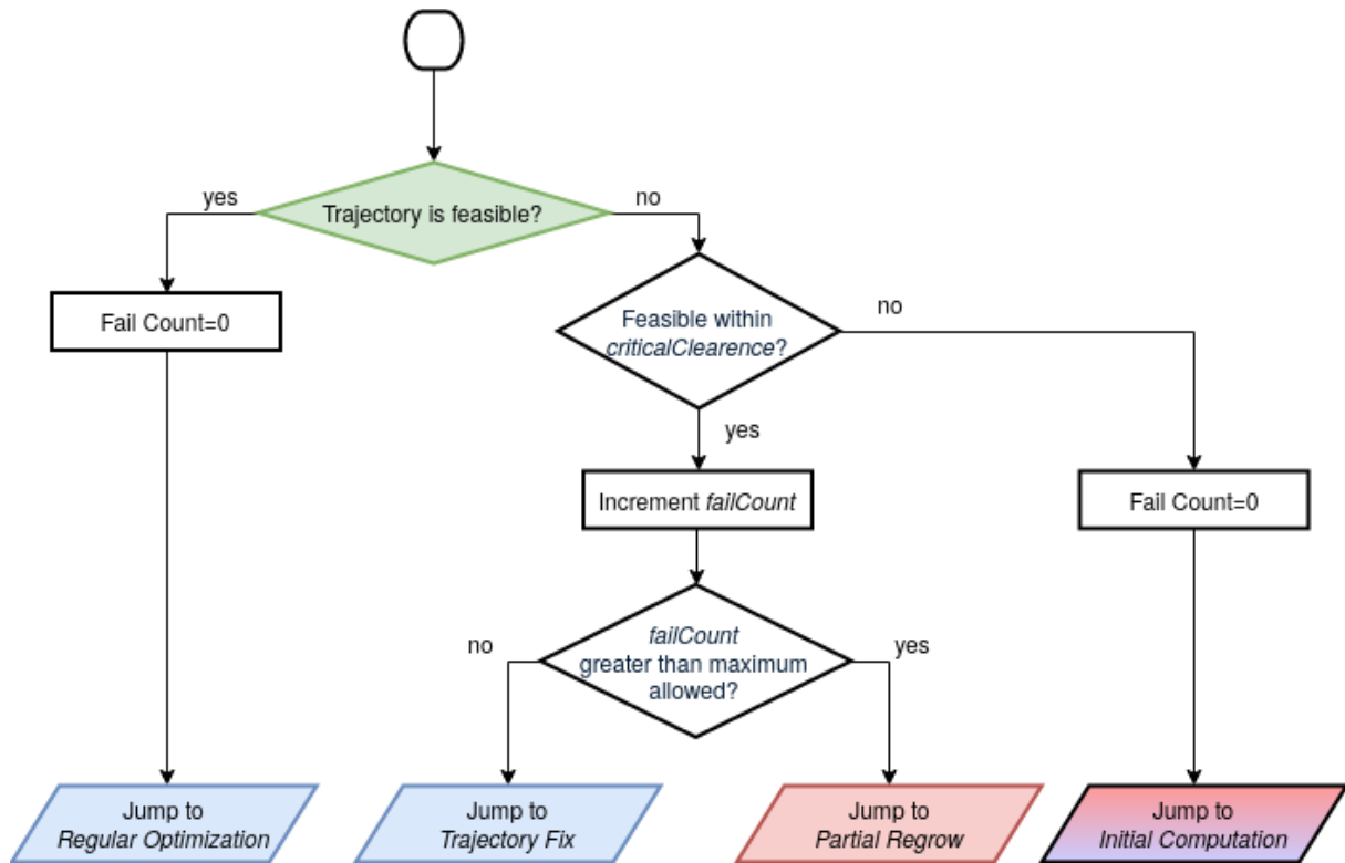
Figure 5.10: Flowchart representing the functionality of the Decision Maker state.
