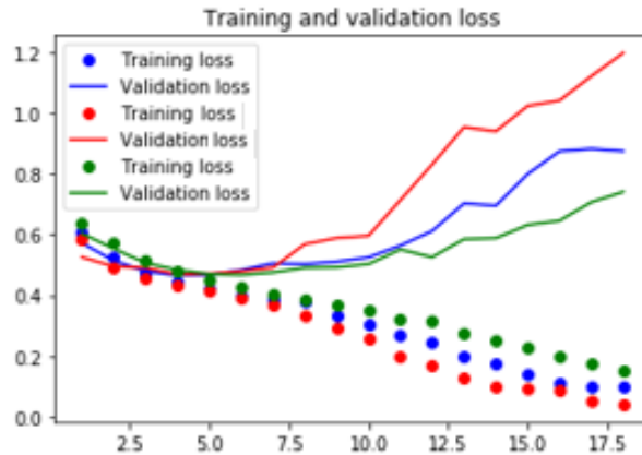
Figure 5.9: Comparison of the validation and training loss curves from training 3 LSTM networks only differing in the number of nodes. Each is composed of 3 LSTM layers with the following number of nodes: red: 512, 256, 128; blue: 256, 128, 62; green: 128, 64, 32.
