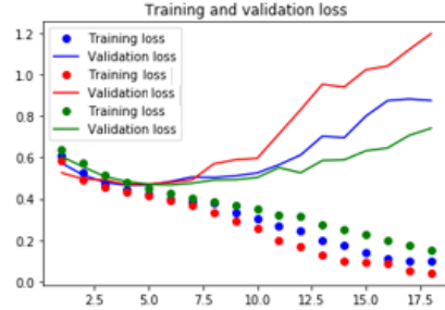
Figure 9: Comparison of the validation and training loss curves from training 3 LSTM networks differing in the number of nodes. Each is composed of 3 layers with the following number of nodes: red: 512, 256, 128; blue: 256, 128, 62; green: 128, 64, 32.
