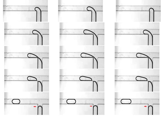
Figure 5: Droplet formation process in the squeezing regime for Q = 0.06, 0.08 and 0.1 (left to right), at Ca = 0.002 , for the T1 geometry.
