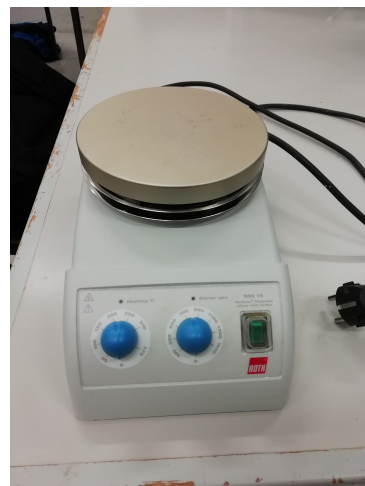
(b) Rotilabo MH15 heating magnetic stirrer from Carl Roth GmbH .
