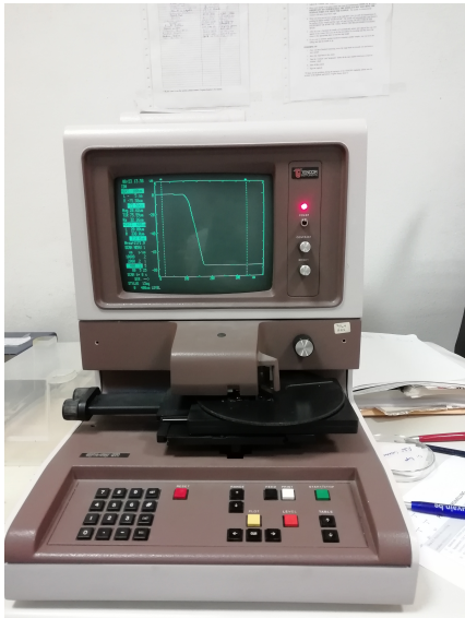
(a) Measurement of SU-8 resist thickness using the Tencor Alpha Step 200 .
