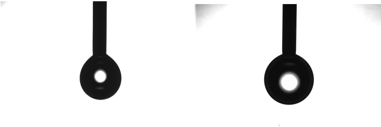
(a) DIW surface tension measurement using pendant drop method. (b) DIW drop formed inside the optical glass cell filled with mineral oil.
