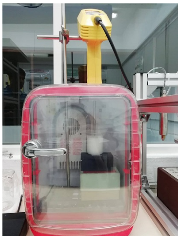
(a) UP200Ht handheld ultrasonic homogenizer from Hirschel Ultrasonics .
