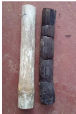
Figure 3: Sample of solid bamboo and the obtained charcoal
