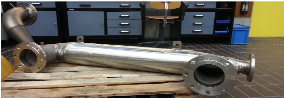
Figure 41 The constructed heat exchanger
