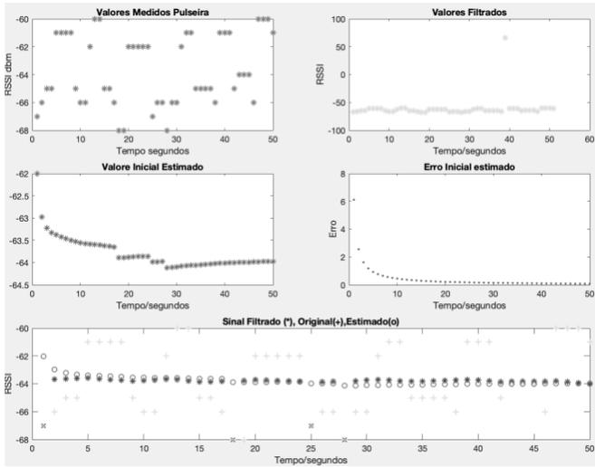
Fig. 1. Operation of the algorithm with values collected at 1 meter between bracelet and a smartphone.
