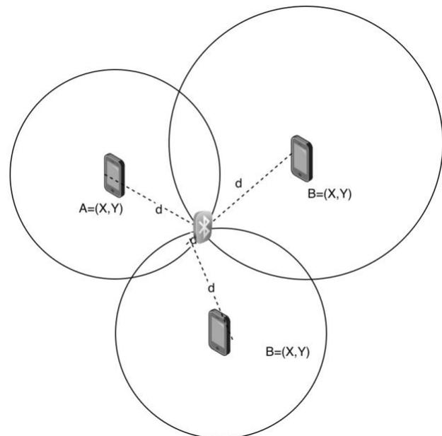
Fig. 3. Trilateration, the d are in meters and the x and y are GPS coordinates, Latitude and longitude. .
