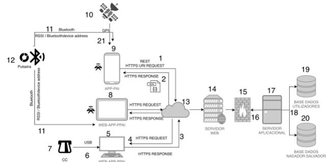
Fig. 2. The proposed architecture for the system PPAI.
