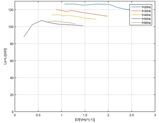
Figure 2-6 - Behavior of the rotor and stator inductance through magnetization levels
