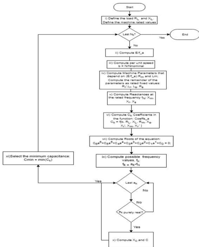
Figure 3-2 - Flowchart of the Matlab analytical Model
