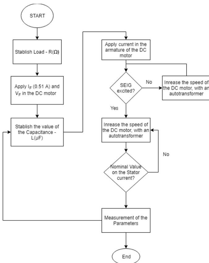
Figure 3-11 - Flowchart of the experimental tests
