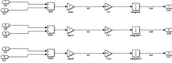
Figure 3-7 - Load block Simulink diagram
