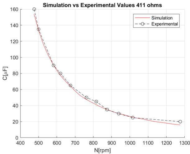
Figure 3-13 - Simulation vs Experimental values for R=411Ω
