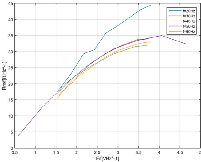
Figure 2-9 - Evolution of the Core losses
