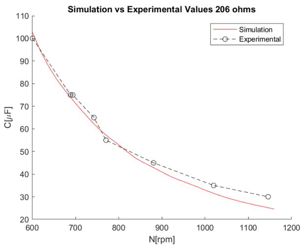
Figure 3-14 Simulation vs Experimental values for R=206Ω
