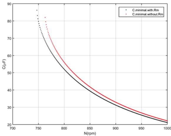
Figure 3-4 - Required minimal capacitances for exciting a SEIG for RL=300
