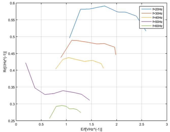
Figure 2-7 - Behavior of the rotor resistance through magnetization level
