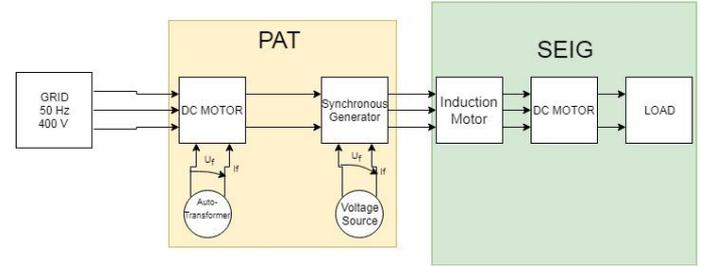
Figure 2-3 - Diagram of the experimental tests for the behavior of the induction machine
