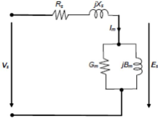
Figure 2-5 - Equivalent circuit for the no-load test adapted from (Paiva, 2011)
