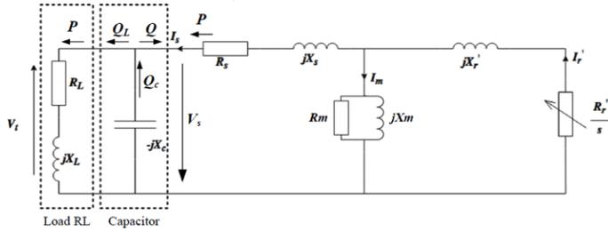
Figure 3-1 - Equivalent electric circuit of the self-excited induction generator connected to the load [(Fernandes et al., 2018)]
