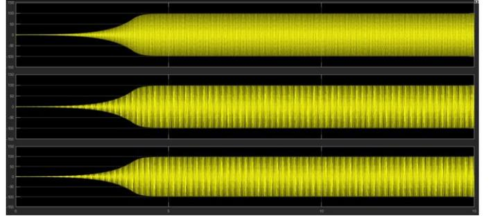
Figure 3-9 - Stator voltage results for a resistance of  $R = 120 \Omega$  and an excitation of  $C = 58 \mu F$  and for a time range of 15 seconds
