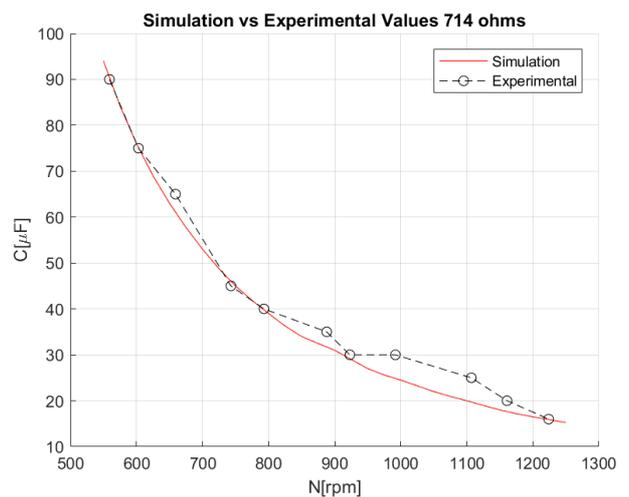
Figure 3-12 - Simulation vs Experimental values for R = 714Ω
