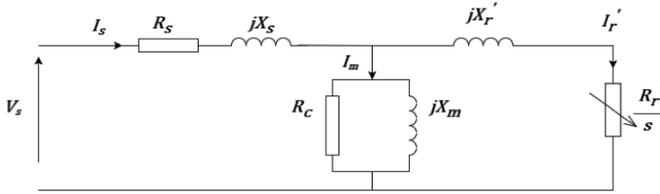
Figure 2-1 – Electrical equivalent of an induction machine
