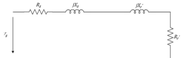
Figure 2-4 - Equivalent circuit of blocked rotor test, adapted from (Paiva, 2011)
