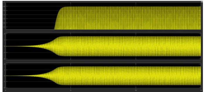
Figure 3-10 - Stator current results for a resistance of  $R = 120 \Omega$  and an excitation of  $C = 58 \mu F$  and for a time range of 15 seconds.
