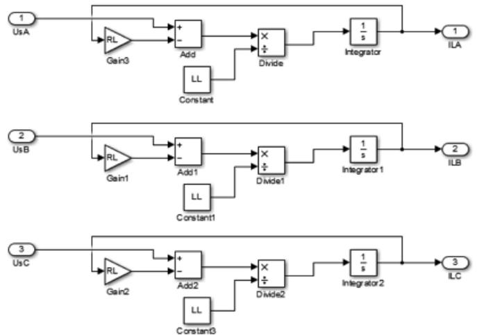
Figure 3-6 - Load Simulink Block Model
