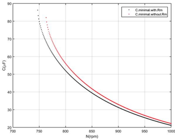
Figure 3-3 - Required minimal capacitances for exciting a SEIG for RL=600
