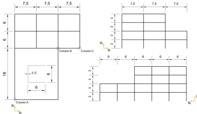
**Figure 7** – Dimensions of the irregular building considered.
