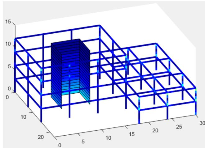
**Figure 9** – Plot showing the amount of mechanical reinforcement ratio after adding a core wall
