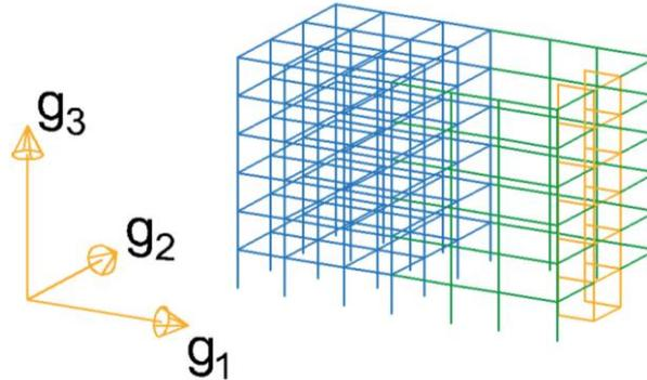
**Figure 1** – Example of a model assembled from the three types of sub-structures considered.
