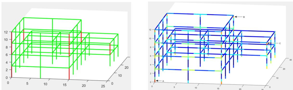
**Figure 8** – Output plots showing the over-stressed elements in red on the left, and the levels of mechanical reinforcement ratio on the right
