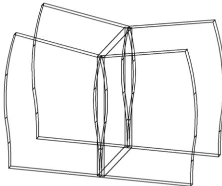
**Figure 3** – Example of an unwanted effect in the regular wall model
