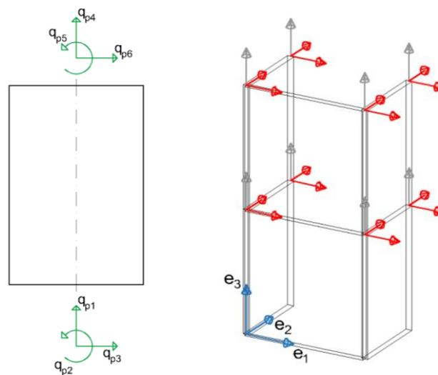
**Figure 2** – Displacements a wall, and distinction between “Slave” and “Local” degrees of freedom in a wall
