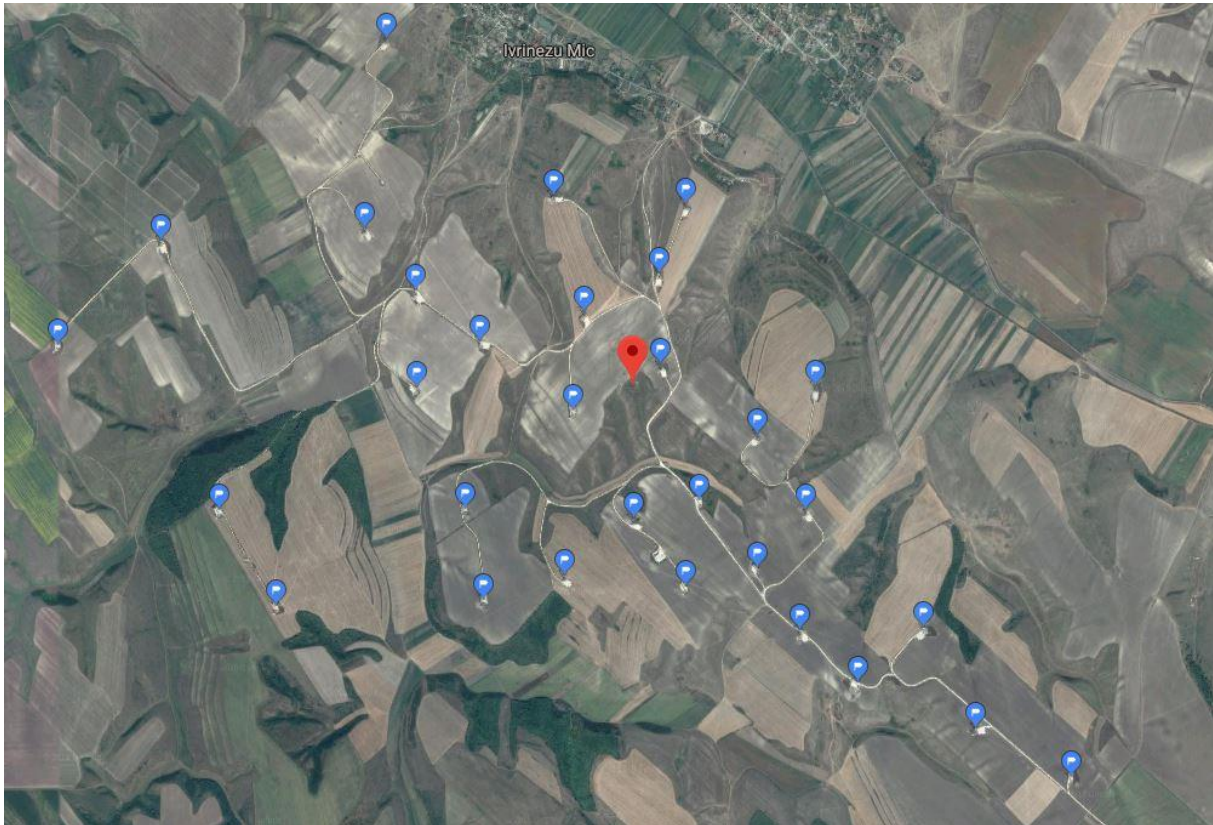
Figure 5 Distribution of wind turbines at the Pestera Wind Farm. Red location indicates the coordinates corresponding to the weather data.
