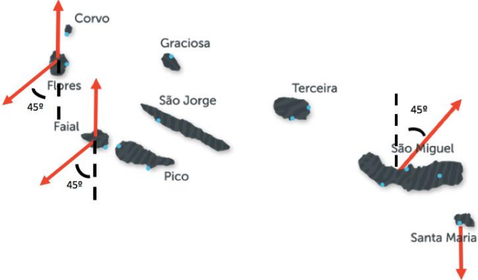
Figure 4-18: 18 elements' Yagi directions of orientation for the 4-frequency system (adapted from [38]).
