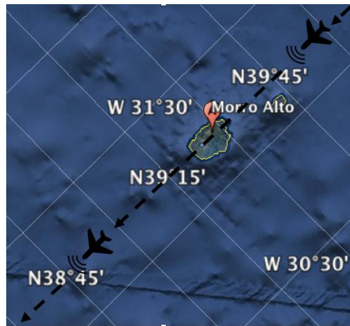
Figure 4-19: Testing aircraft's route from NE heading SW for the Morro Alto, Flores, Ground Station.
