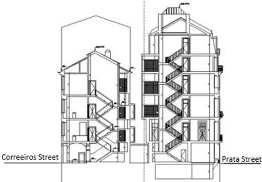
Figure 2 – Cross section throughout the buildings before the rehabilitation works.
