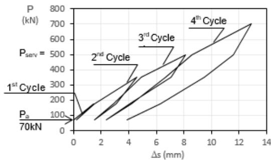
Figure 13 – Load-displacement curve of the load test
