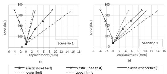
Figure 14 – Graphic of elastic and plastic displacements and elastic limits of the free length for both scenarios.
