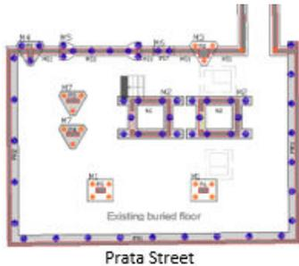
Figure 4 - Designed foundations plant for Building 1 (JETSJ, 2016).
