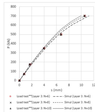
Figure 18 - Load test simulations through Plaxis 2D
