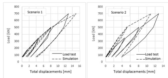
Figure 15 – Load test simulation for both scenarios.
