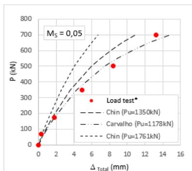
Figure 16- Simulations of the load test  $K_E=0,4$  (Fleming method).
