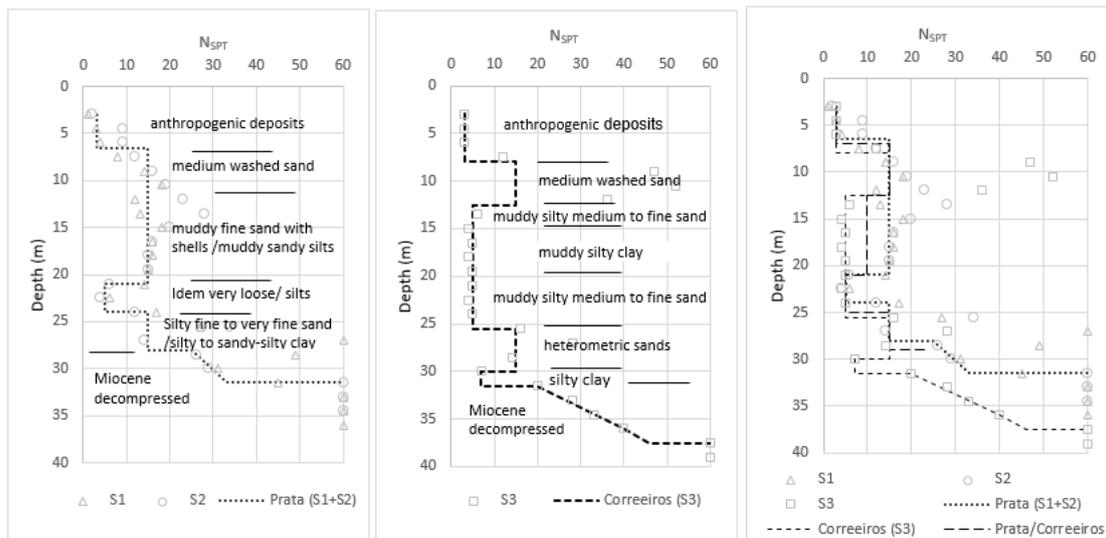
Figure 7 - Graphic of SPT values vs. depth and estimated type profiles.
