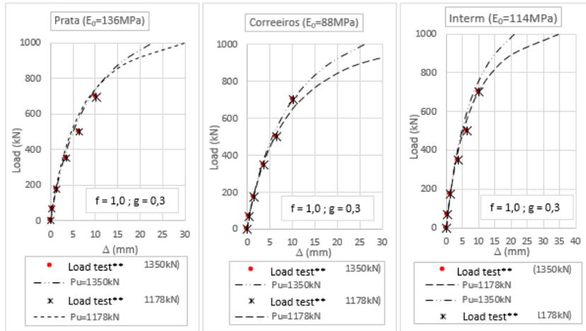
Figure 17 - Load test simulations (Mayne and Schneider method).
