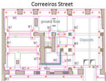
Figure 3 - Designed foundations plant for Building 2 (JETSJ, 2016).
