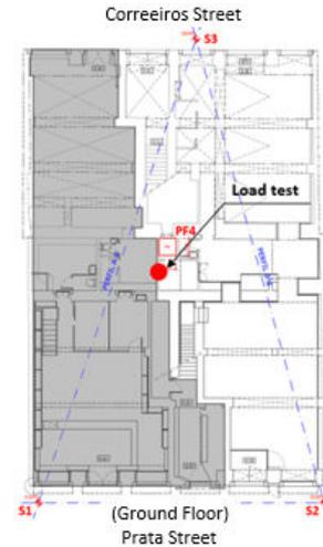
Figure 6 - Spatial distribution of geotechnical boreholes and approximate location of the load test
