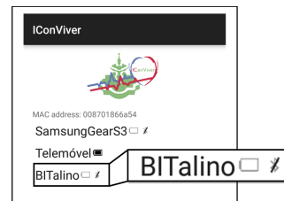
(c) Display after information from the server is received. BT symbols indicate there is still no connection with the other devices.
