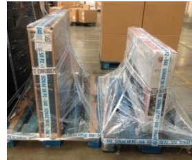
Figure 4 Two cases of inefficient consolidation of pallets
