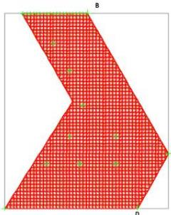
Figure 10 - Slab band model in SAP2000, for basements -3 and -5
