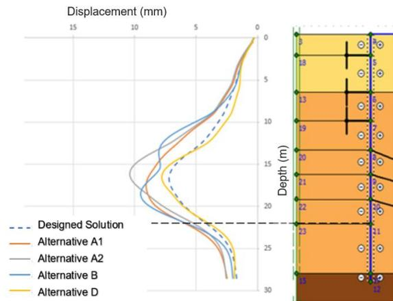
Figure 16 - Comparison of the displacements in the earth retaining structures of piles in the DE elevation, transversal to the tunnel of the Marquês, buried
