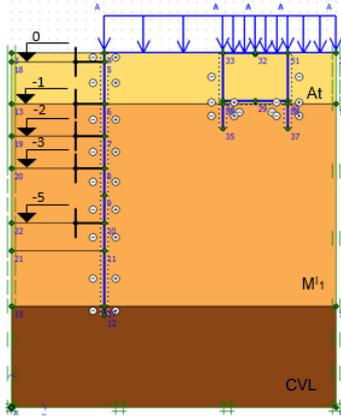
Figure 8 - Cross sections in the DE elevation, transverse to the tunnel of the Marquês, underground
