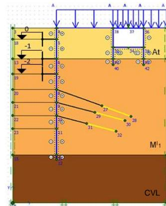
Figure 7 - Cross sections in the DE elevation, transverse to the tunnel of the Marquês located on the surface
