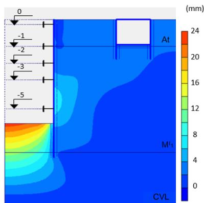
Figure 113 - Total displacements associated to the initially design solution of the cross section in the DE elevation, transversal to the tunnel of the Marquês, buried
