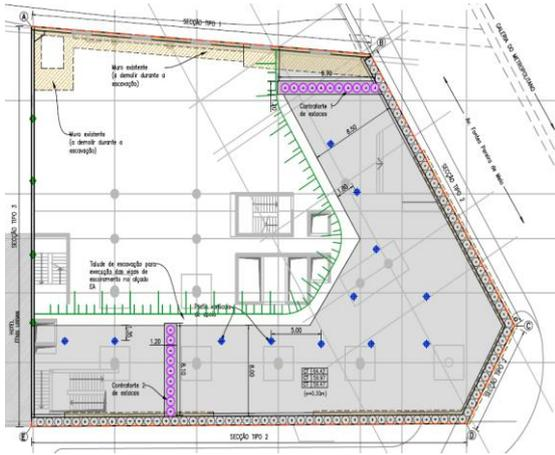
Figure 3 - Plant of the design solution for basements 0, -1 and -2 (A Pinto & Pita, 2016)
