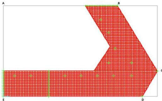
Figure 9 - Slab band model in SAP2000, basements 0, -1 and -2
