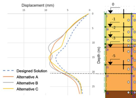
Figure 14 - Comparison of displacements in the piled earth retaining structures in the BC elevation, transversal to the ML tunnel
