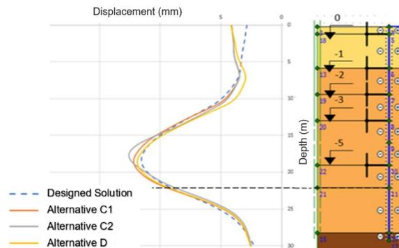
Figure 15 - Comparison of the displacements in the piled earth retaining structures in the elevation DE, transversal to the Tunnel Marquês located at the surface
