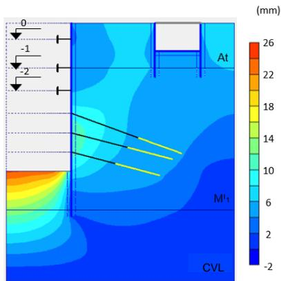
Figure 102 - Total displacements associated to the initially design solution of the cross section in the DE elevation, transversal to the tunnel of the Marquês located on the surface
