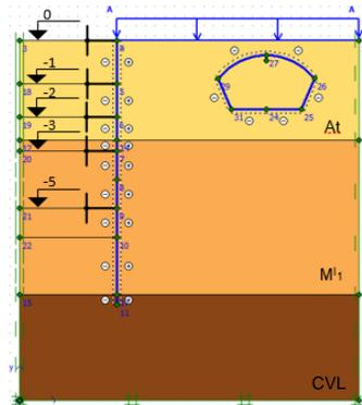
Figure 6 - Cross section in the BC elevation, transverse to ML tunnel
