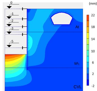
Figure 11 - Total displacements associated with the solution initially designed for the cross section in the BC elevation, transversal to the ML tunnel
