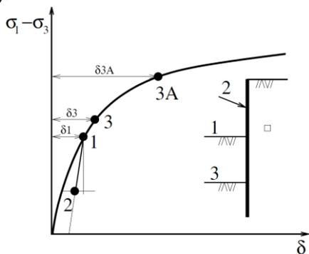
Figure 1 - Schematic representation of the evolution of the stresses state in ground elements supported by anchored earth retaining structures, (Guerra, 2007)
