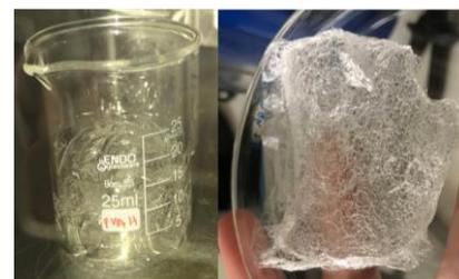
Figure 3: Extreme removal of oxygen: vacuum made water come to a boil and air bubbles solidified onto the gel.
