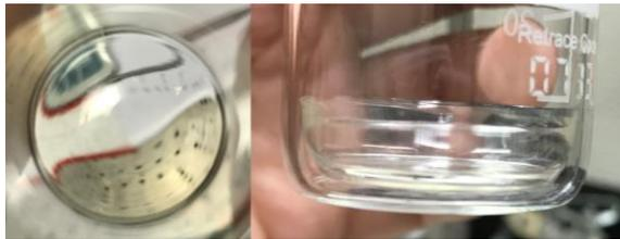
Figure 5: Thin PVA hydrogels: up and side views.
