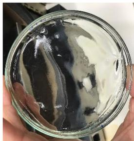
Figure 6: Thick PVA hydrogel.
