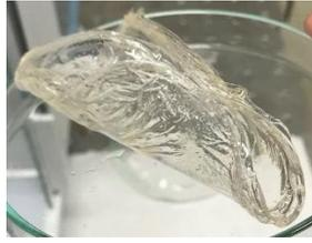
Figure 4: Semi irreversible contracture of thick PVA hydrogels.
