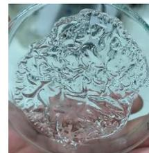
Figure 2: Striations of the gel upon rapid cooling and oxygen exposure of the pre-gel solution.
