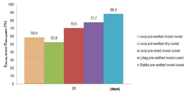
Fig. 3 - Relation between SLWAC and NWC for splitting tensile strength at 28 days
