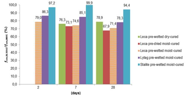
**Fig. 2 - Compressive strength of SLWAC relative to NWC**
