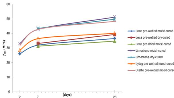
**Fig. 1 - Concrete's compressive strength evolution over time**
