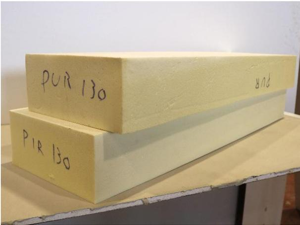
**Fig. 1:** Blocks of rigid PUR and PIR foams used at experimental campaign.
