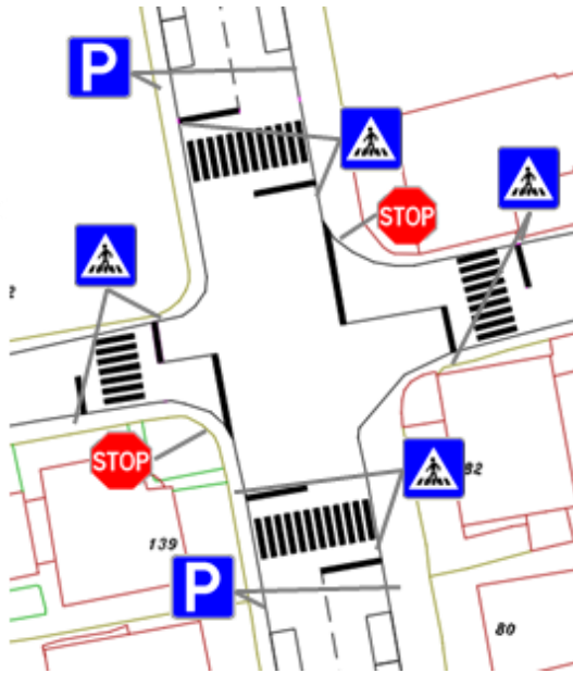
Fig.9: Example of some corrective measures proposed, in this case, for the intersection between Avenida Liberdade and R. Alexandre Robalo Cardoso
