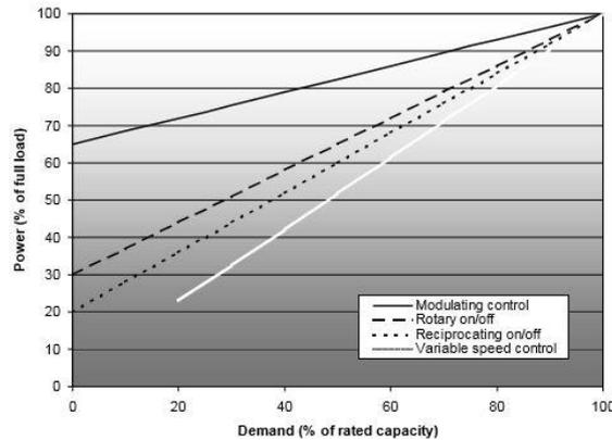
Figure 4 - Power (% of full load) variation with demand (% of rated capacity) in a constant torque load machine, with different flow control mechanisms (4).
