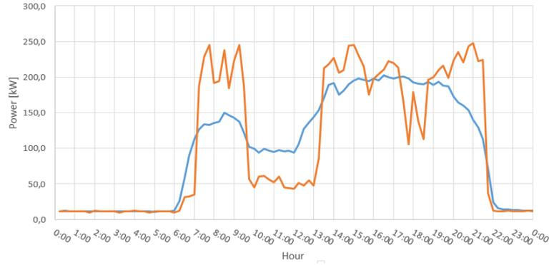
Figure 2 – Daily Load Profile (the red curve represents a typical day and the blue stands for an average profile)
