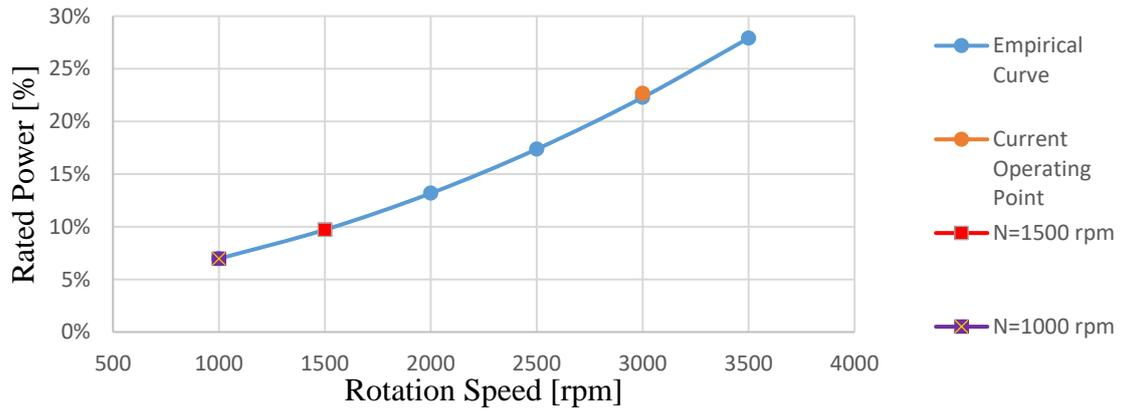
Figure 3 - Empty hammer mills empirical power curve and operation points before and after VSD installation (N = 1000 rpm and N = 1500 rpm)
