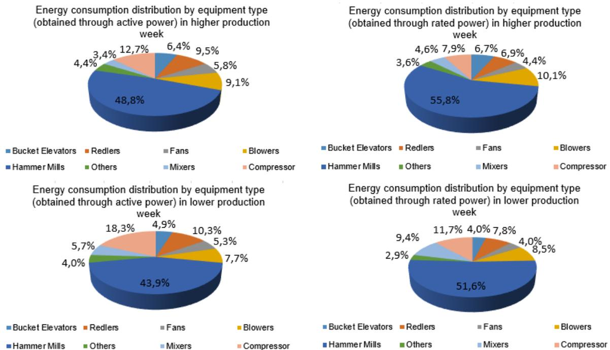
Figure 1- Energy consumption distribution by type of equipment
