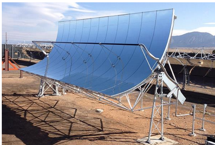
Figure 2 Concentrator with parabolic trough [12]
