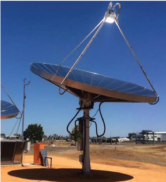
Figure 5 Concentrator with parabolic dish[14]
