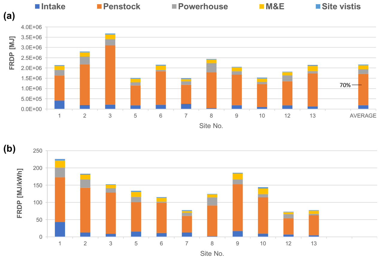
Figure 4.10. Breakdown of fossil resources depletion potential by components of each MHP project (a) expressed as MJ (b) expressed as MJ/kWh.
