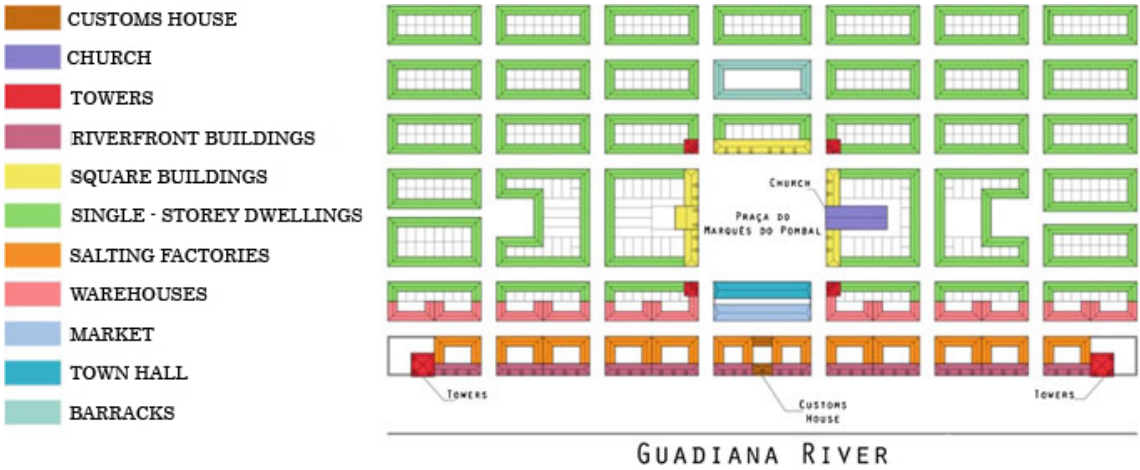
Figure 2-23 - Original plan of Vila Real de Santo António and main building types (Picture from Ortega et al. [25])
