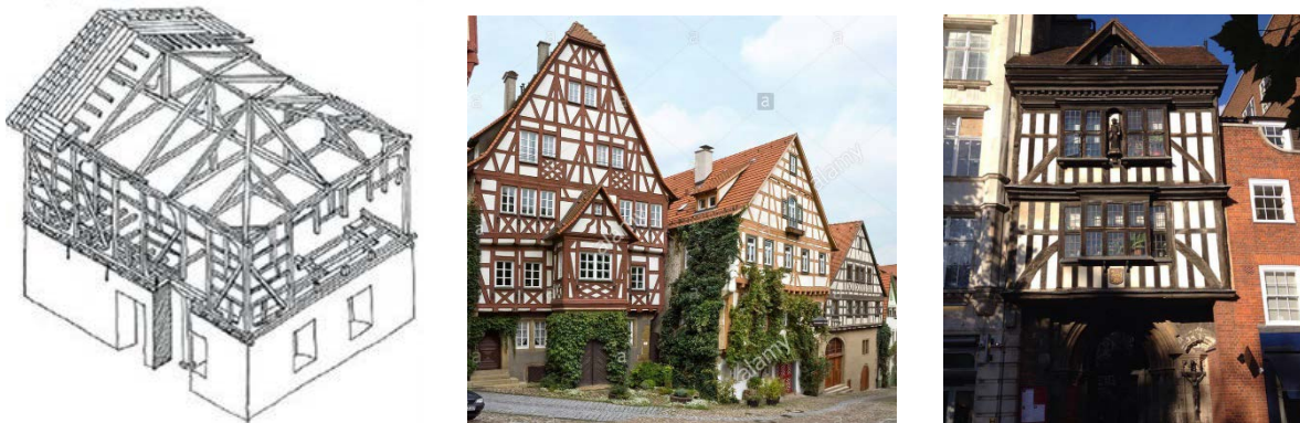
Figure 2-28 - Timber-frame houses: in the left typical house of Lefkada Island (Greece), on the centre the houses in the medieval town of bad wimpfen in baden wuerttemberg, on the right St Bartholomew Gatehouse, built in 1595 in London
