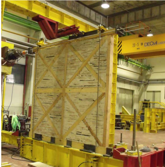
Figure 2-26 – a) Final layout of the experiment with load cell, LVDT and jacks; b) Schematic of the “frontal” wall specimen (units in meters otherwise specified) (Pictures extracted from H. A. Meireles PhD Thesis in Civil Engineering, 2012, [16])
