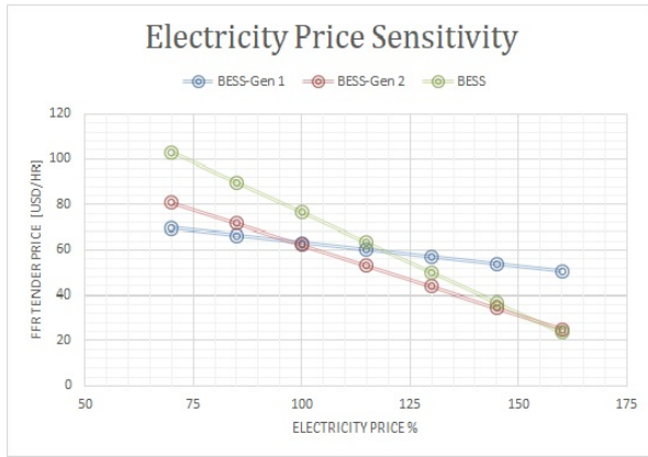
Figure 7: Sensitivity analysis to examine how percentage variations in the electricity price (100% is present value) determine the FFR tender fee for each plant
