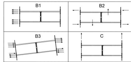
Figure 2.4: Bridge crane horizontal reactions
