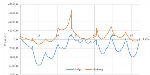
Figure 4.3: BMD along the beam for the SLS
