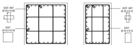
**Figure 4.12:** Reinforcement of columns
