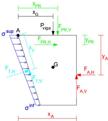
Figure 3.2: Acting Forces on cross-section
