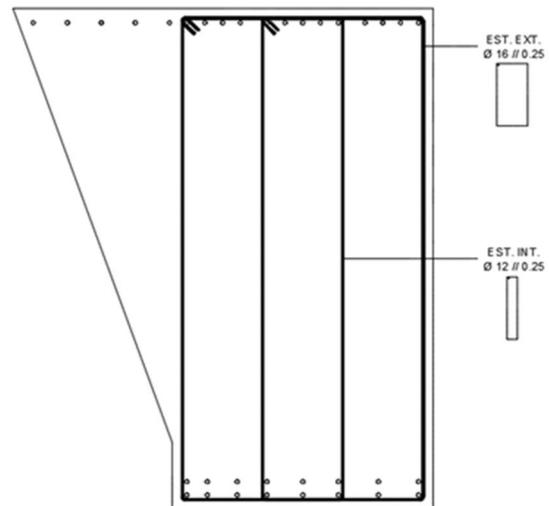
**Figure 4.8:** Transverse reinforcement
