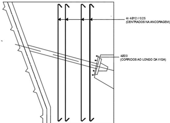
Figure 3.5: Reinforcement in the Anchorage zone
