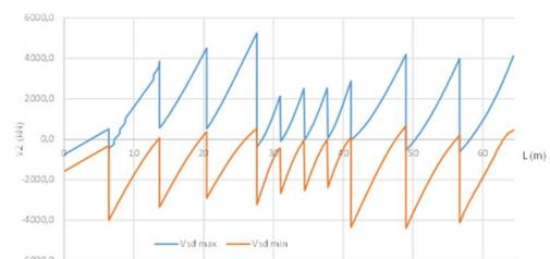
Figure 4.4: SFD along the beam for the ULS
