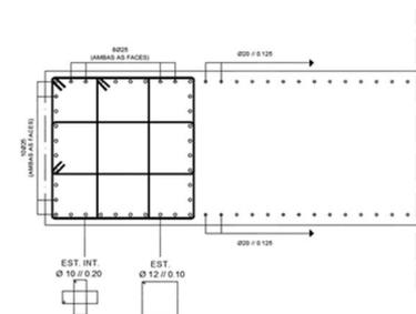
**Figure 4.13:** Wall reinforcement (Stirrups not represented)
