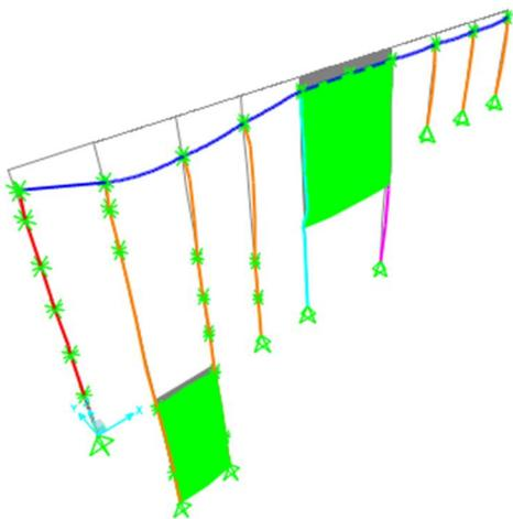
**Figure 4.9: Deformation for the SLS**
