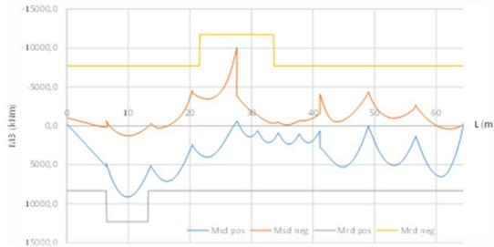
**Figure 4.7:** Resisting bending moments for ULS
