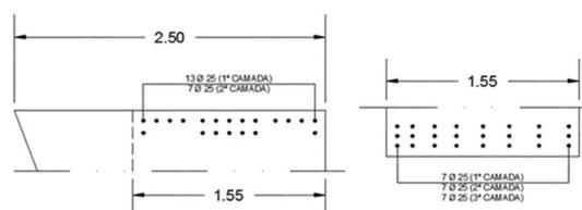
**Figure 4.5:** Reinforcement bars for bending moment
