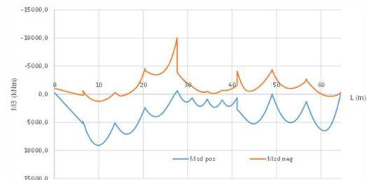
Figure 4.2: BMD along the beam for the ULS
