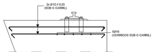
**Figure 4.10: Reinforcement under the bridge crane**
