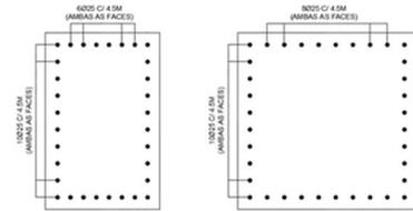
**Figure 4.11:** Columns longitudinal reinforcement (stirrups not represented)
