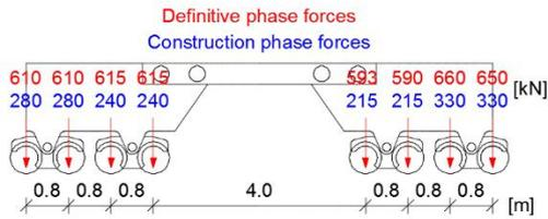
Figure 2.2: Bridge crane and vertical forces
