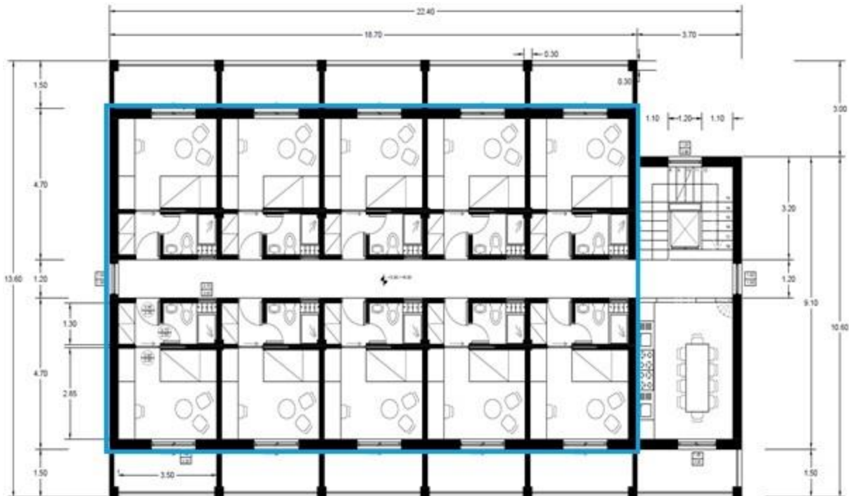
Figure 2: The insulation (blue) and corresponding thermal-conditioning zone.
