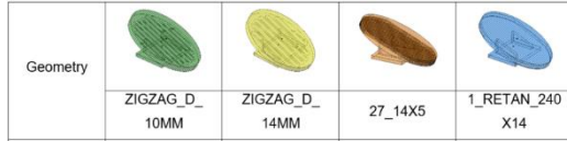
Figure 11 - Cooling channel geometries for the receiver mirror.
