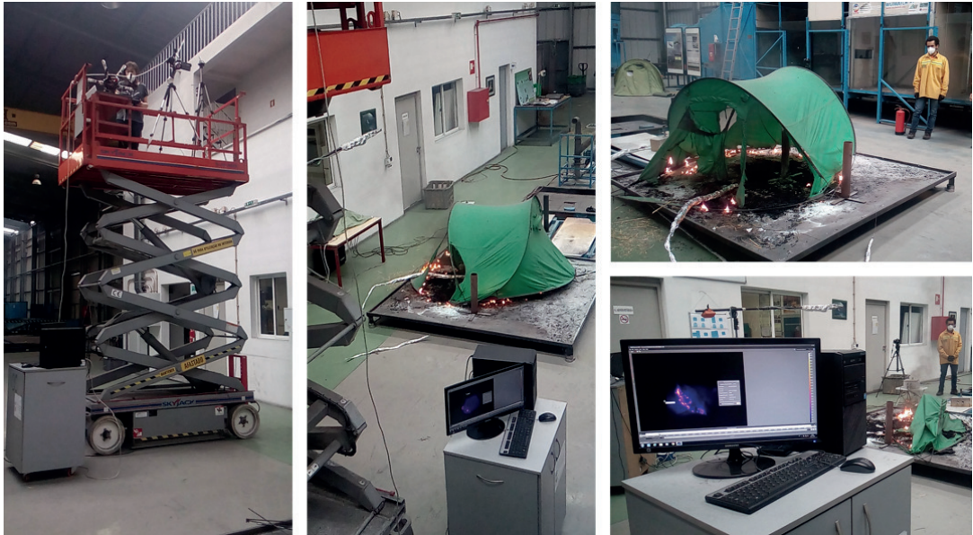
Figure 2.9: Experimental setup for the burning of a tent.
