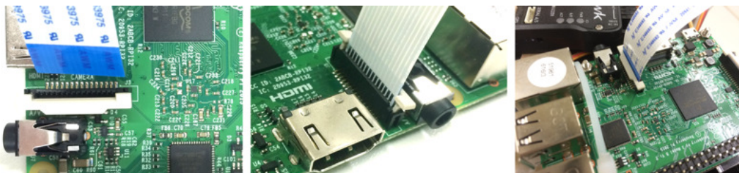
Figure 2.4: Installation of Raspberry Pi Camera Module V2.
