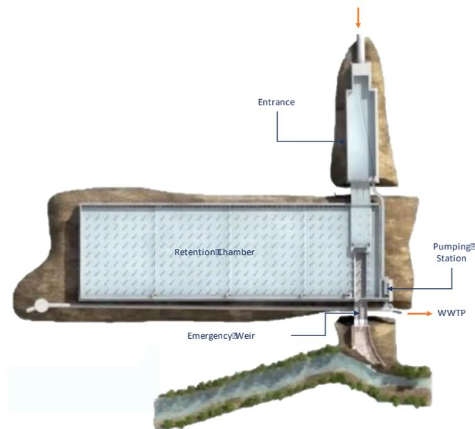
**Figure 1** – Schematic representation of a storage basin.
