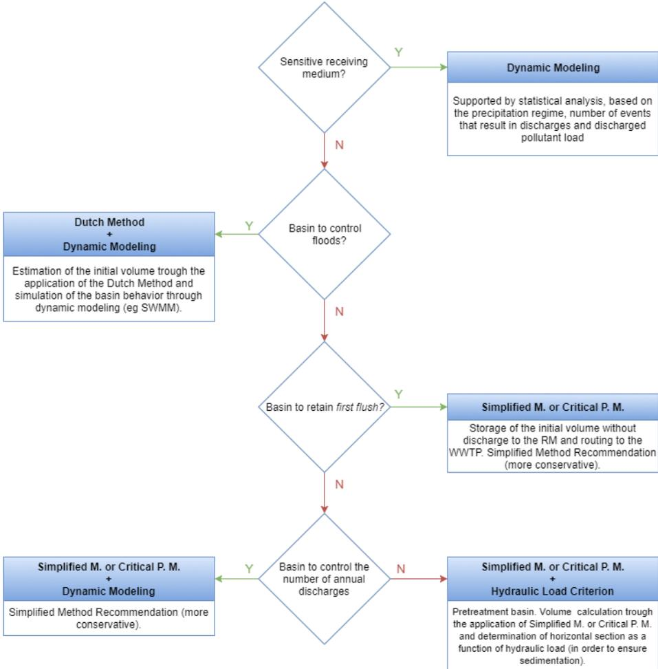
Figure 2 - Flowchart of the designing processes according to the purpose of the storage basins.
