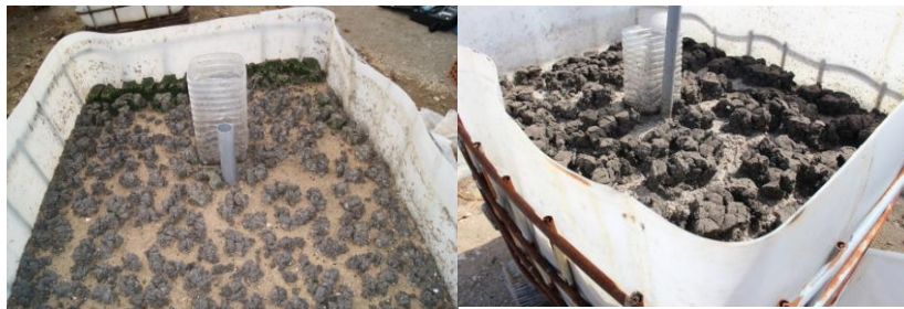
Figure 4 - Clumps formed by cracking and retraction of sludge
