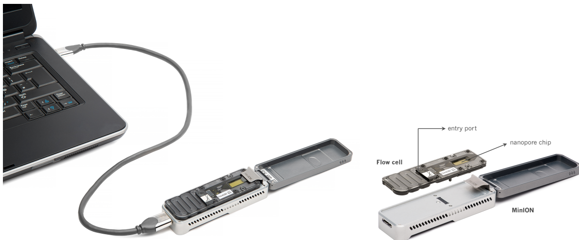
Figure 2.3.2.1 | MinION set-up. The disposable flow cell is mounted into the MinION and the device is then connected by a USB 3.0 cable to a computer with the MinKNOW control software. This figure is an adaptation of the original pictures made available by Oxford Nanopore Technologies.
