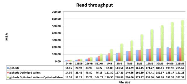
Figure 12: gipherfs optimizations: impact on read throughput
