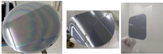
Figure 2 From left to right: porousified 8inch wafer, free-standing epifoil (19 cm diameter), bonded epifoil (11cmx11cm) on a glass substrate.
