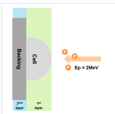
Figure 3.2 illustration of the geometry used in the analysis. Proton (P) beam striking a sample (Cell), deposited onto a 1.5 µm polycarbonate foil (Backing). The cell and the backing are independent layers of analysis (see text for more details).
