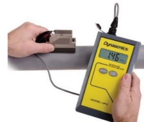
Figure 4 – Ultrasonic Flow Meter (Mitchell Instrument Company Inc.®, 2014).
