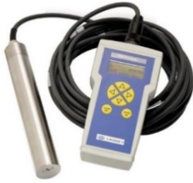
Figure 6 – Portable TSS meter (Hach, 2015).
