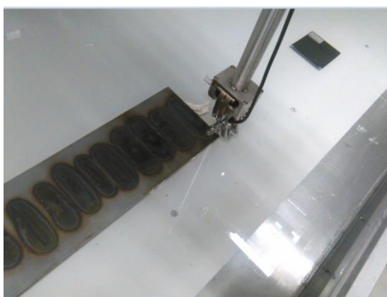
Figure 3.12: Experimental procedure equipment for the Phased Array test, where the plate is submerged and the scanning probe is coupled with the automated system.
