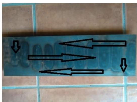
Figure 3.13: Trajectory made by the sound probe in the Phased Array ultrasonic testing
