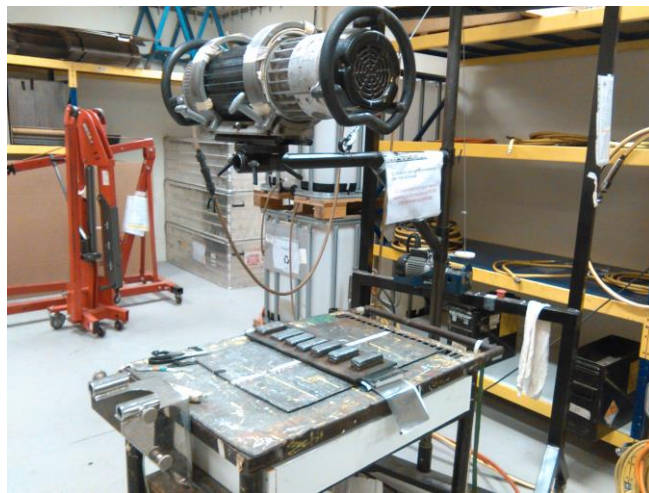
Figure 3.14: Experimental setup for the radiation NDT
