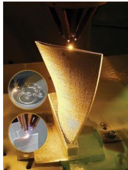
Figure 2.13: Manufactured part and processing using LENS technology [39]
