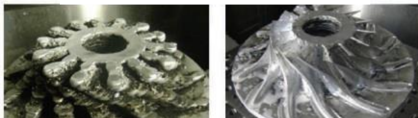
Figure 2.17: WAAM manufactured part before machining (left) and after machining (right) [39]
