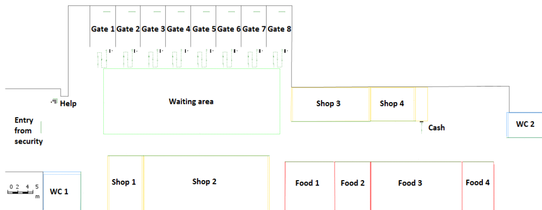
Figure 2. Plan of the terminal 2 of Lisbon airport in the developed model on AnyLogic
