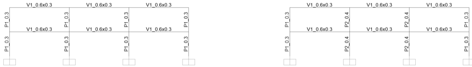
Figure A.12 – Model M_A.II_R for x=0m and x =28m (left) and for x=7m, x=14m and x=21m (right)
