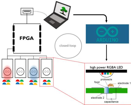
**Fig. 1 Schematic of the OptoPAD** From the FlyPAD on the left to the clockwise direction we find the PC running Bonsai and receiving the capacitive data stream; Bonsai is able to send activation messages to different pins of the Arduino (the actuator), which will activate the different colours of the LEDs on top of the FlyPAD behavioural arenas where the animals are interacting with food.
