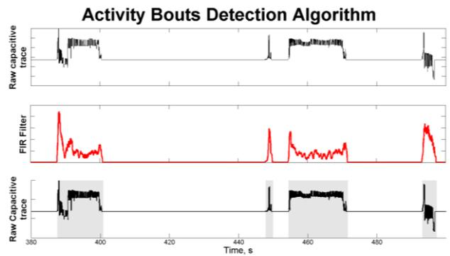
**Fig. 3 Activity Bouts Detection Algorithm** The first plot shows a detail of the raw capacitance signal of a fly interacting with food; the second is the same signal depicted previously already processed by the algorithm until the FIR filtering (derivative, absolute value and FIR filter); the final plot represents the same capacitance signal with the grey shadows identifying activity bouts.
