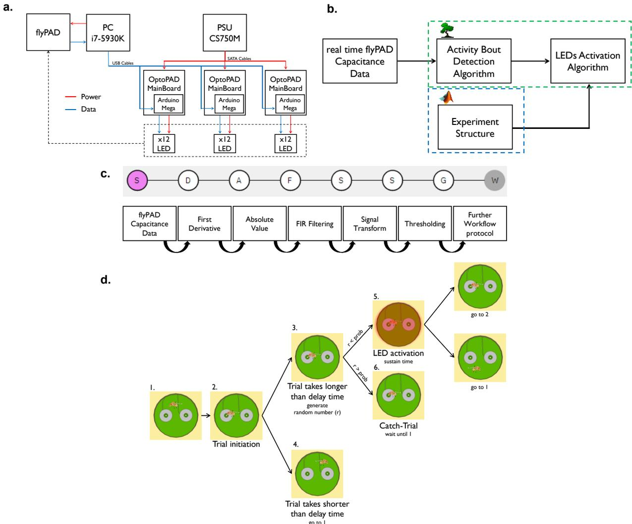
**Fig. 2 Hardware and Software** **a.** Complete hardware system schematics; **b.** Data flow in the complete OptoPAD system; **c.** Bonsai: Activity Bout Detection Algorithm; **d.** Experiment structure: 1. Fly walks in the arena; 2. Fly finds a food source; 3. Fly keeps interacting with food for longer than the “delay” time; 4. Fly does not interact with food for longer than the “delay” time; 5. LED is active for “sustain” time; 6. Catch-Trial: system waits until the activity bout is over
