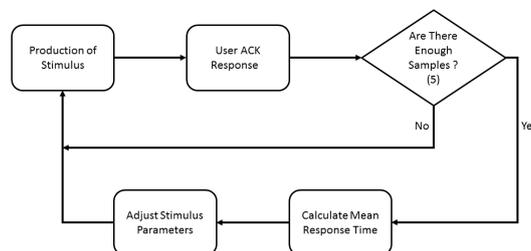
**Figure 4:** Flowchart for the closed chain feedback in the Attention Monitor feature.
