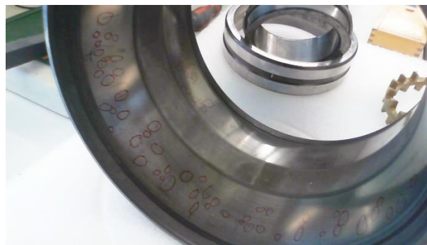
Figure 7: Typical defects on a bearing outer raceway.
