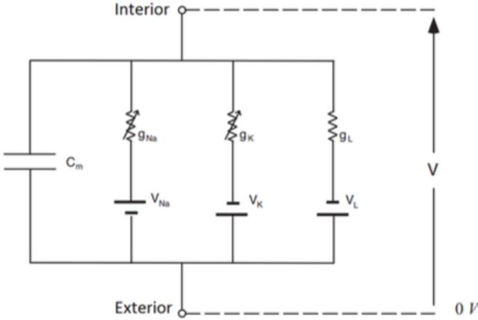
Figure 2: Equivalent electrical circuit of the cell membrane (Hodgkin and Huxley, 1952). Each branch of the electrical circuit represents the contribution to the total transmembrane current from a specific ion specie channel. In this case, three different type of ion channels are embedded in the cell membrane,  $Na^+$ ,  $K^+$  and a leakage  $L$ .
