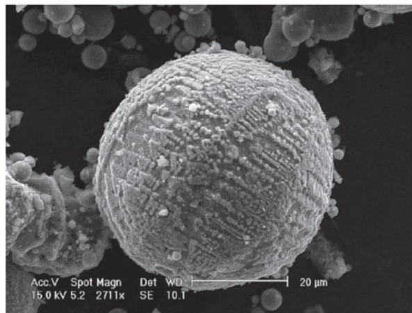
Figure 19 SEM image for magnetic sphere in fly ash [36].
