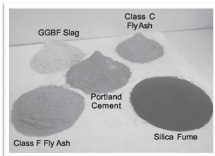
Figure 11 Comparison of fly ash class F and C, Portland cement, silica fume and GGBF slag [45].
