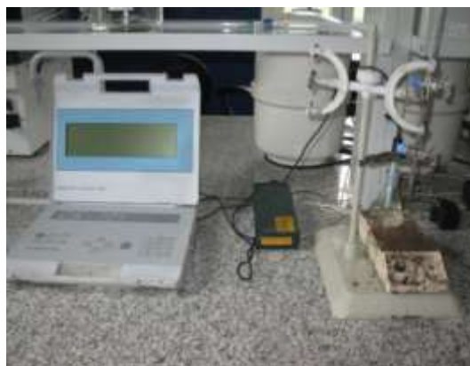
Figure 28. Apparatus for potentiometric titration for determining of chlorine content.
