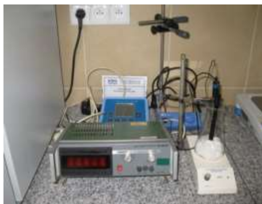
Figure 29. Apparatus for potentiometric titration for determining of fluorine content.
