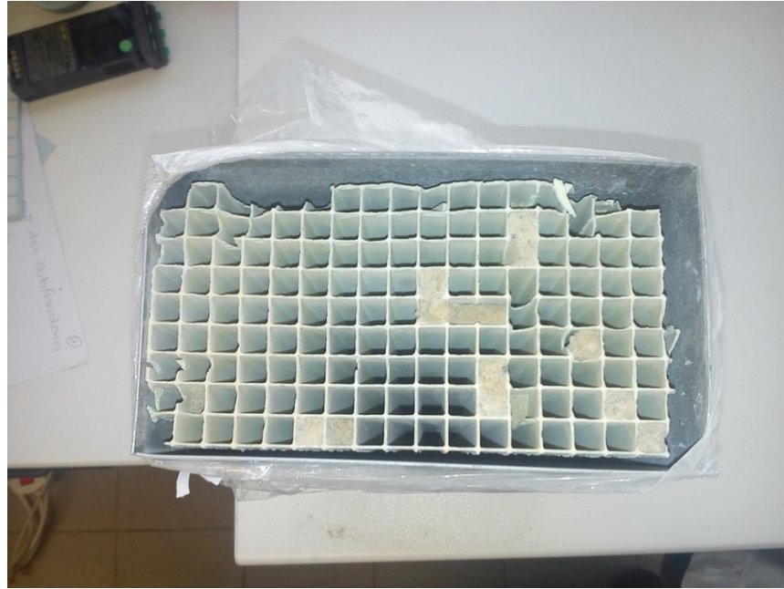
Figure 9 The catalyst monolith in steel casing after exposure to flue gas for 9405 hours
